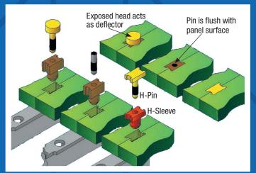
H-Pin and Sleeve Systems lock adjacent panels together, resulting in superior hold-down forces.
